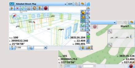
MAGNET Field is a powerful and intuitive field application software that enables you to collect survey mapping data and perform construction and road layout using total stations, levels, GNSS receivers and GTL-1200.
