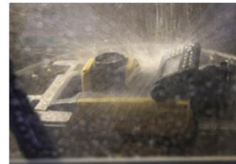
We perform the tough environmental tests to ensure long-term operation even under the rough site environments.
