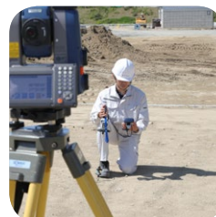
Auto-tracking test under high speed vibration conditions
