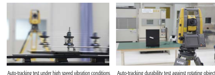
Auto-tracking test under high speed vibration conditions Auto-tracking durability test against rotating object.
