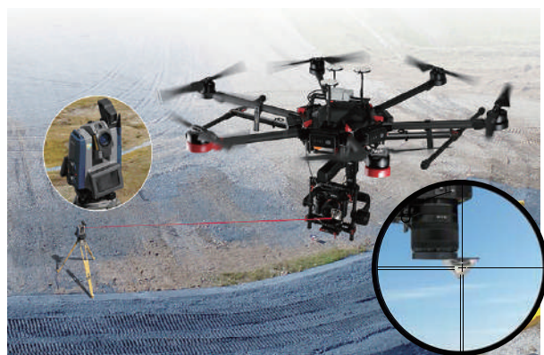
DRONE ROBOTIC STATION
